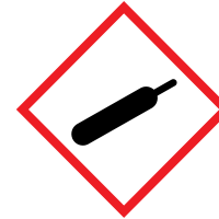
GAS UNDER PRESSURE
